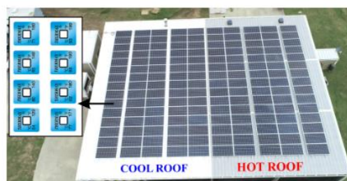
Figure 5 THERMAX technique (Thermax®) for thermal evaluation of the Rubicon buildings' roofs. [34]
